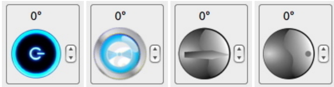
Figure 13: Container RoundButton . You can change the angle with the UpDownArrow control, the circular button by the mouse. The appearance of the container can be set and the user may create its own logos.
